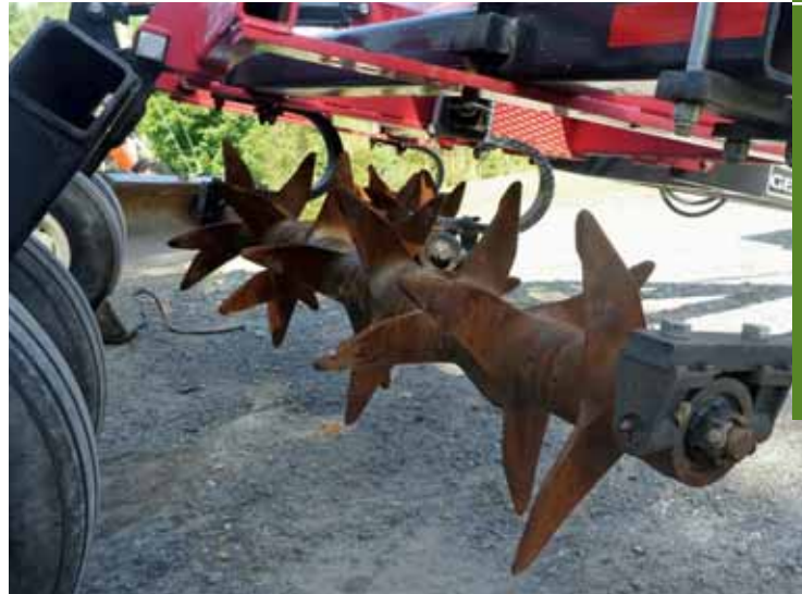
Above, left: Aerator slits in annual crop land. Right: Tines on an aerator cut into compact soil and incorporate liquid on annual crop land.
