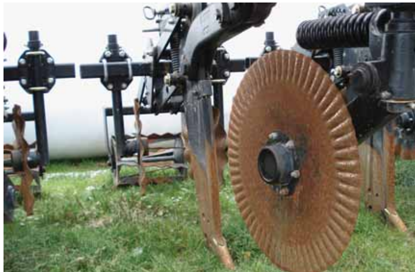
Above, left: A corn grain field after using a tillage machine creates a seed bed. Right: A Zone Builder tillage machine. The front disk cuts through residue, an adjustable shank breaks through different lengths of compacted soil layers, and the rolling basket in the rear breaks up soil clods.
