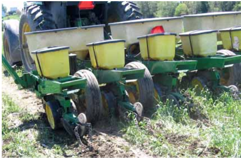
Above, left: Ryegrass planted with a no-till seeder. Right: A no-till seeder being used to plant a field.
