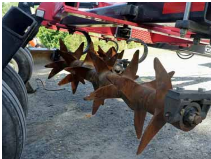
Above, left: Aerator slits in annual crop land. Right: Tines on an aerator cut into compact soil and incorporates liquid on annual crop land.
